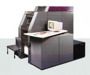
(That's short for Heidelberg Quickmaster DI - the Direct Imaging Printer - featuring computer-to-press simplicity, allowing short runs as small as 100 pieces, and eliminating all those extra manual steps involved in regular offset printing)
